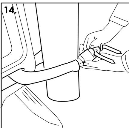
14. Place the chain through one the holes at the bottom of the body and around the post/wall fixing bracket. Secure in position.
