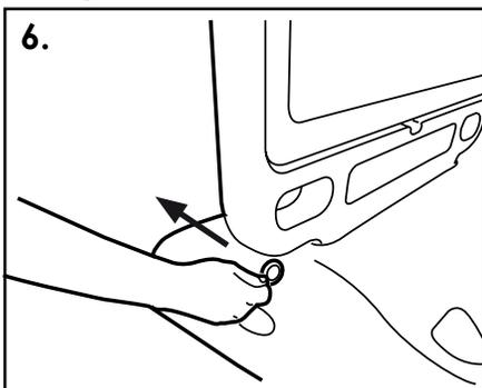
6. To fill with water, remove the filler cap on the side of the base. Ensure base is on a flat surface.
