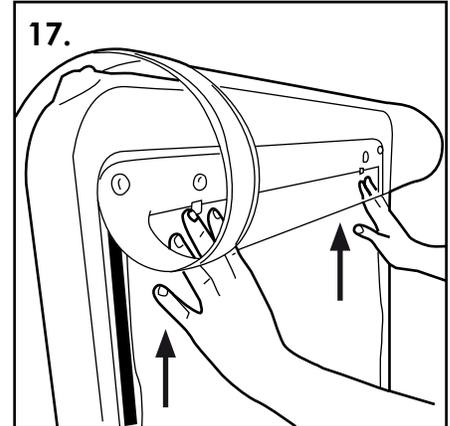
17. Take the poster and push the top edge underneath the two poster clips until it stops so that it is held securely in place. Ensure that both side edges of the poster are overlapping the magnets on the body.
