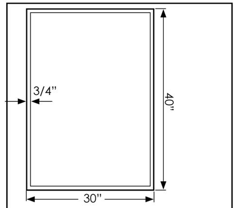
The unit is designed to frame a 40 x 30 inch poster. The poster can either be printed on paper or it can be laminated for added durability. NOTE: The clear polycarbonate protector has a printed border therefore the graphics must be inset so they are not hidden by the border. See dimensions above.
