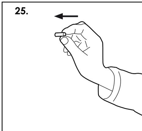
25. Insert a wall plug into each hole and lift the unit back into position on the wall.
