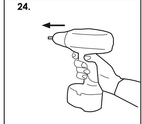
24. Remove the unit from the wall and drill 4 off holes where the markings appear on the wall.
