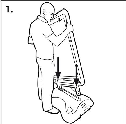
1. Place empty base on the ground and locate the two body legs into the slots within the base.
