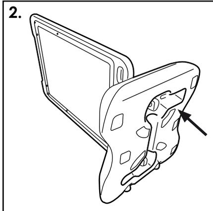
2. Tilt the unit and lay on its side in order to gain access to the underneath of the base.
