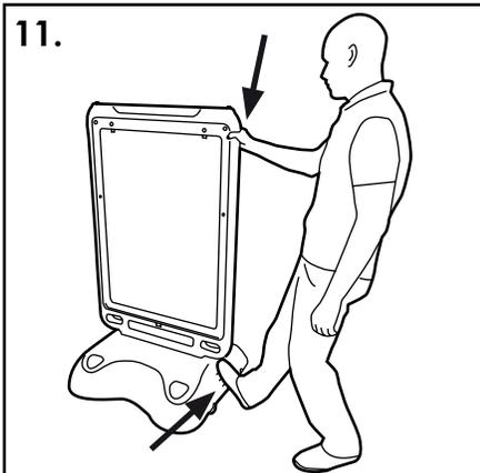
11. Place hand(s) around the side of the body and place your foot on the foot rest detail on the side of the base.
