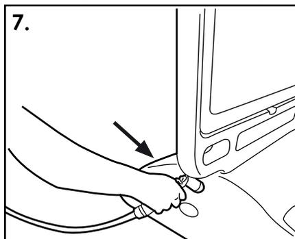
7. Using a hose fill the base until water reaches the filler hole. DO NOT over fill as there will be no space for expansion if the water freezes.
