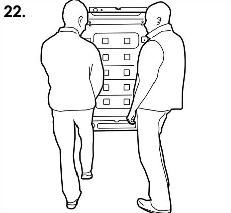
22. Lift the unit and position where suitable on the wall using a level to ensure it is horizontal. NOTE: the rectangular personalisation recess should be at the bottom.
