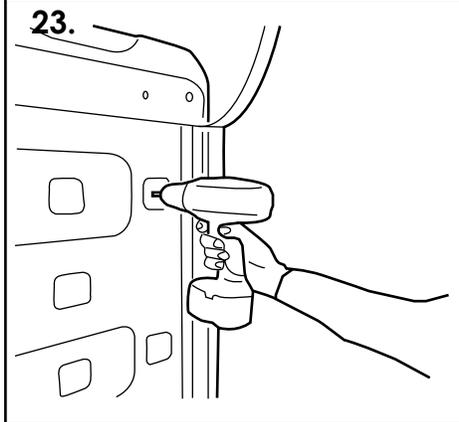
23. Open the clear polycarbonate cover by lifting upwards. Using a 7mm or 8mm masonry bit, drill through each of the 4 holes in the unit to make a small mark on the wall.
