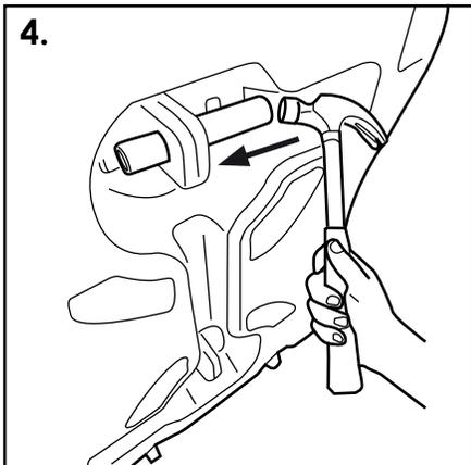
4. Using a hammer, tap the peg through the leg until it snaps in place (overrides lip) and locks.
