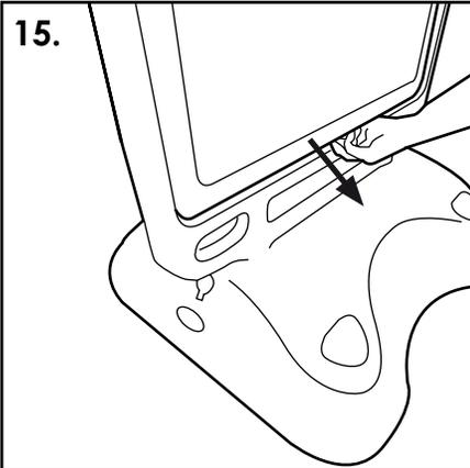
15. Place fingers into the opening recess at the bottom of the body and pull the clear polycarbonate protector away from the body/magnets.
