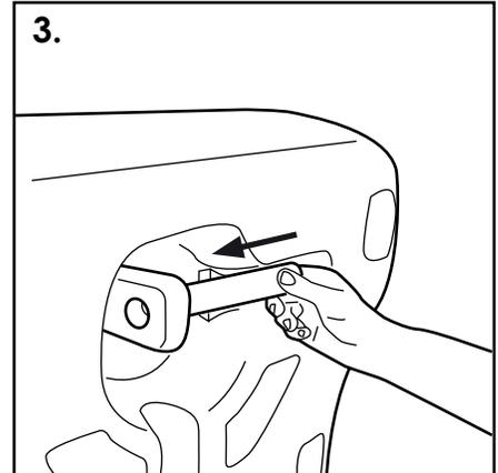
3. Taking one of the two pegs provided insert the rounded end first into one of the holes in the body leg.
