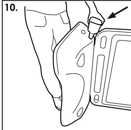
10. Using a funnel, pour sand through filler port until it reaches the level of the filler hole.
