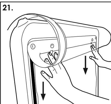
21. Pull the poster downwards from underneath the poster clips to remove. Unclip the clear protector from the press studs and pull back down into position over ensuring all the magnets are connected.
