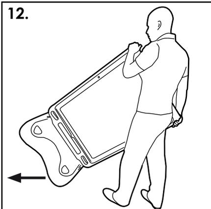
12. Using your foot and hands to lever the unit, tilt the unit towards you so that the wheels engage with the ground. Push the unit to its location.
