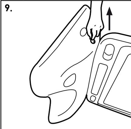
9. To fill with sand, lay the unit on its side in order to gain access to the fill port and remove filler cap.
