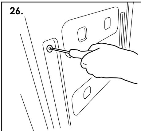
26. Place a 25mm washer onto a 60mm screw provided and push through hole in the unit. Place a 28mm spacer onto the screw so that is located between the unit and the wall. Locate the screw with the wall plug and fix the unit to the wall using a pozi drive screwdriver. Repeat on remaining 3 off fixing points. DO NOT overtighten.
