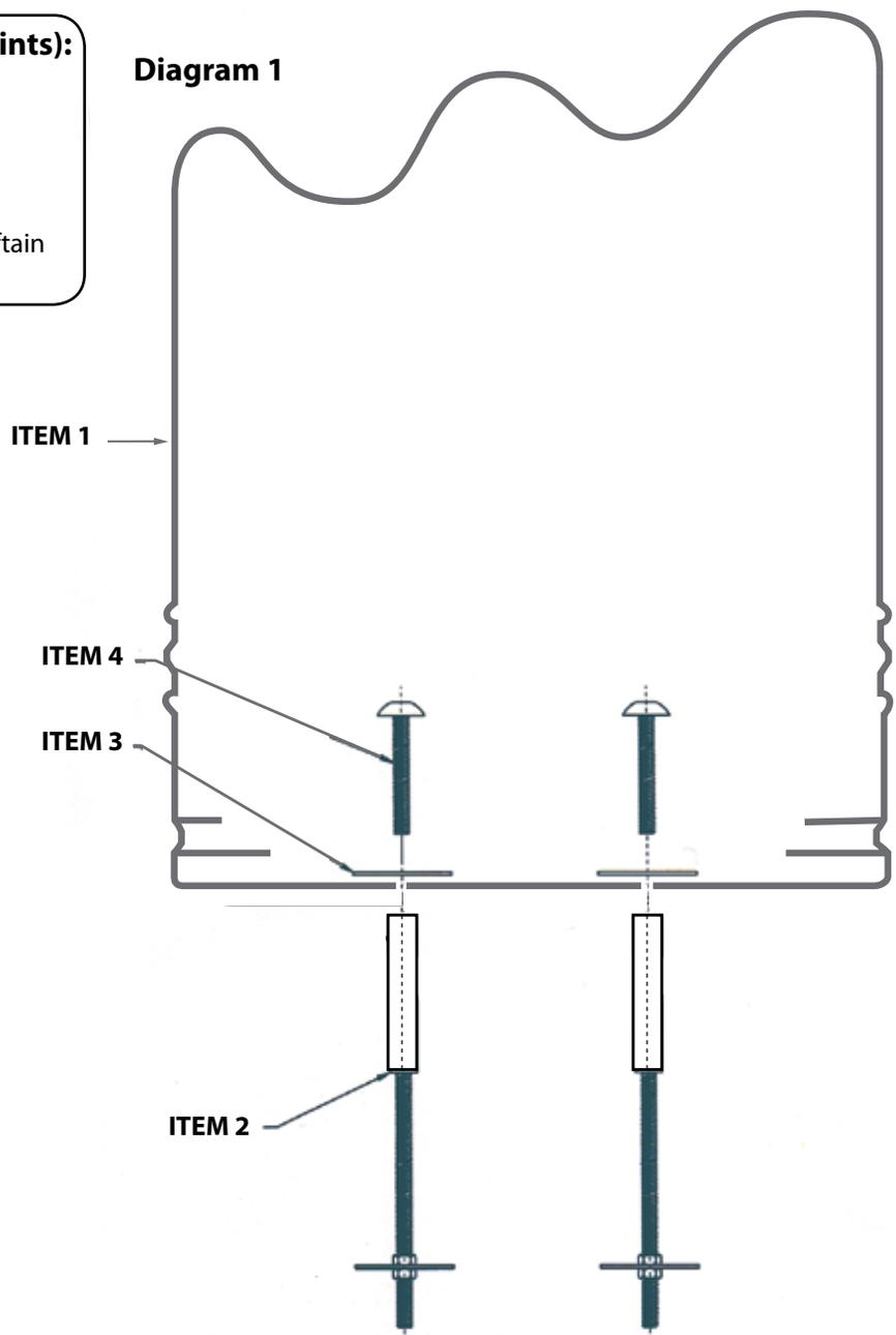
6. Remove the unit and fixing assembly and pour the concrete mix into the prepared hole up to ground level.
