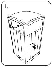
Insert the Glasdon triangularshaped key provided into the keyhole on the side of the unit.
